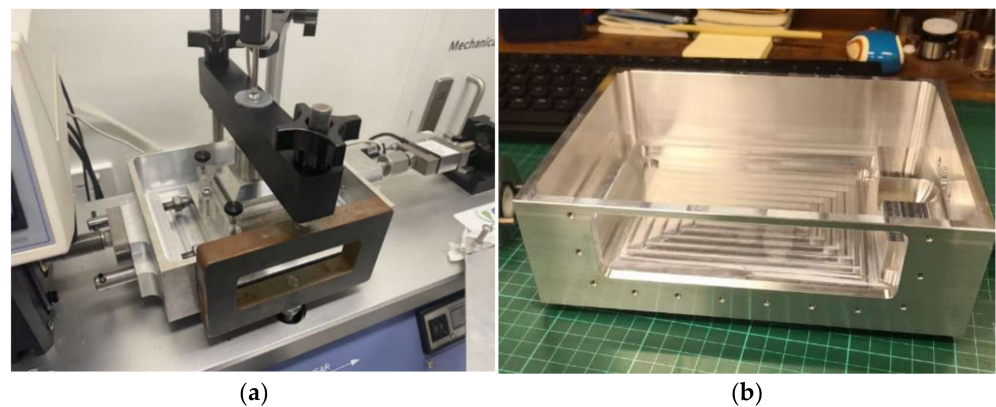
Figure 19. Custom-made (a) modified loading frame and (b) modified water chamber by the authors for preliminary interface shear study.
