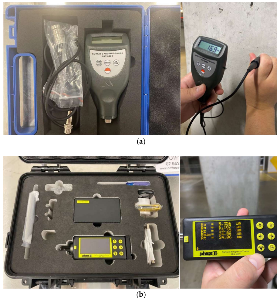
Figure 9. Portable surface roughness gauge: (a) surface profile gauge (large range and low resolution); (b) surface roughness gauge (low range and high resolution).
