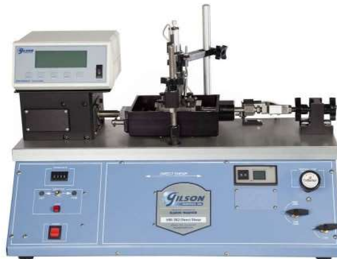
Figure 1. Direct shear test apparatus (HM-382F) produced by Gilson company. This original direct shear apparatus has since been modified by the authors for use as an interface shear apparatus.
