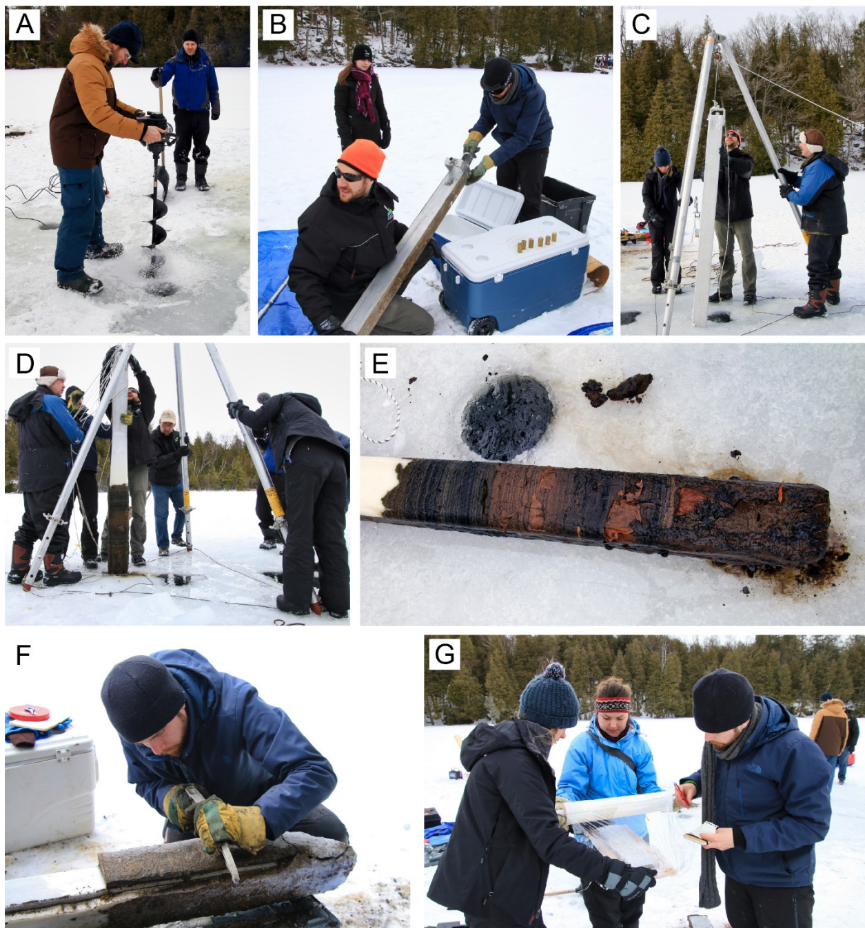
Figure 3. 2019 Coring at Crawford Lake. (A). Creating a hole in the ice for the coring device to be lowered through the water column to the lake bottom. (B). Filling freeze corer with a slurry of dry ice (solidified carbon dioxide) and ethanol. (C). Corer is lowered through the water into the sediment water interface. (D). Freeze core is pulled back up to surface. (E). The corer laid out on the ice, metal side up, which under the winter conditions permitted the sediments to continue to solidify while photos and core logging took place. (F). Core being cleaned and sectioned for transport. (G). Sectioned core segments were laid on labeled boards and wrapped before being placed in dry ice packed coolers for transport to Carleton University.
