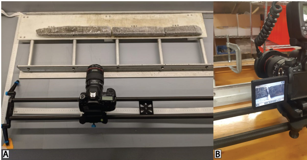
Figure 4. (A). Photography set up showing camera mounted on sliding rail to image a cross section of the core. (B). Ring light mounted on camera.
