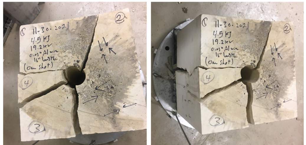
Figure 9. Limestone sample: 0.76 mm wire diameter, 0.5 g weight, and 4.5 kJ discharge energy.
