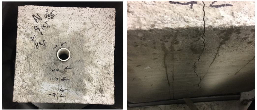
Figure 8. Cement sample: 1.5 mm wire diameter, 0.5 g weight, and 9 kJ discharge energy.
