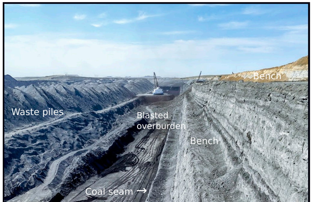
Figure 3. Removal of overburden and waste rock generation during open-pit coal mining at the Cordero Rojo Mine, Powder River Basin, Wyoming, USA.
