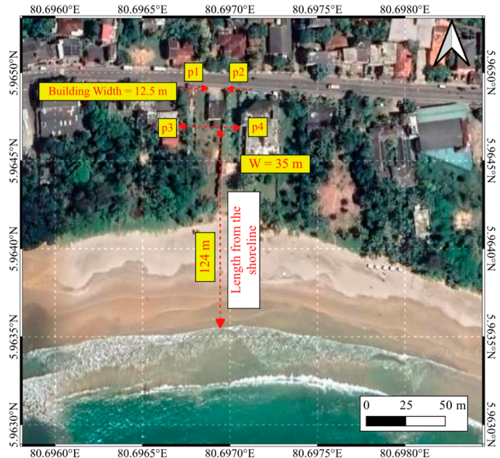
Figure 1. The satellite image depicts the selected b_B/W = 0.36 in an actual scale, located in Dickwella, Matara, Sri Lanka: 12.5 m is the actual building width ( b_B ); 35 m is the approximate channel width ( W ); p1 and p2 are the sides of the building selected; p3 and p4 are the points on the adjacent structures, which represent the flow channel width.
