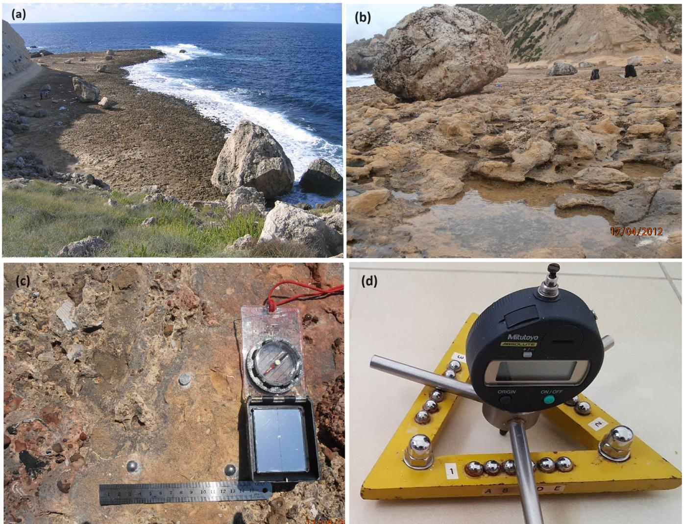
**Figure 2.** (a) Shore platform surface at Ponta tal-Qammieh, Marfa Ridge; (b) Conglomerate Bed (C1) known as Qammieh Bed; (c) MPQ1 TMEM bolt site; (d) Mitutoyo Traversing Micro-erosion Meter.
