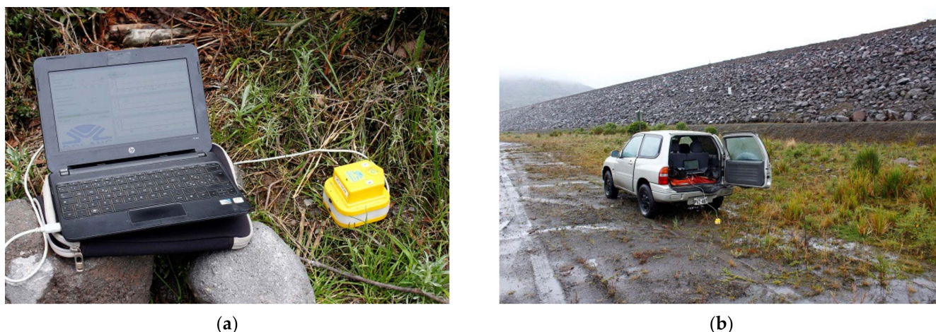
Figure 4. Detailed view of the measurement equipment installed on the ground recording the #4 HVSR station (a). The #8 research point with the equipment measuring and the view of the dam's downstream side in the image's background (b).
