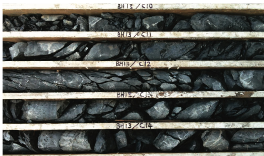
Figure 1. Phyllite cores collected from soil investigation represent low RQD [11].
