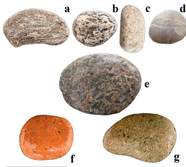
Figure 8. Typical aspect and composition of the main pebbles and cobbles forming the beach deposits. (a) Gneiss (Sample TB11). (b) Augen gneiss (Sample TB11). (c) Granitoid (Sample TB11). (d) Quartz (Sample TB11). (e) Dark grayish sericitic phyllite with randomly oriented post-kinematic andalusite porphyroblasts (Sample TB13). (f) Pinkish porphyroid clast (antique pink type color, Sample TB12). (g) Light grayish porphyroid clast (Sample TB12). Scale bar: 5 cm.
