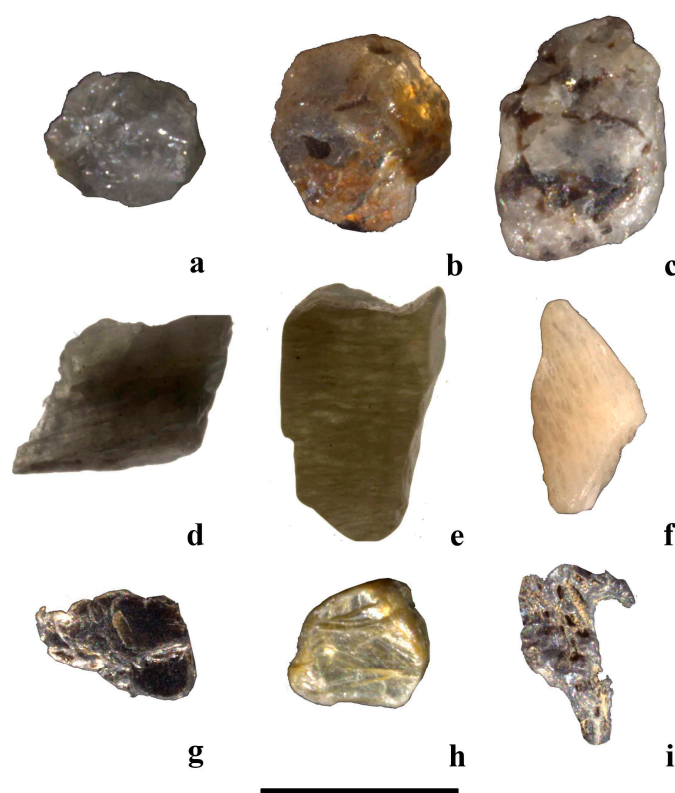
Figure 4. Main types of mineral grains forming the sands (Sample TB01, 1–2 mm sandy fraction), observed under stereomicroscope. (a) Quartz. (b,c) Polyminerals grain of quartz + feldspar + biotite gneiss (b) and augen gneiss (c). (d–f) Monomineralic grain of feldspar showing typical cleavage, and pinkish color in (f). (g) Monomineralic grain of biotite showing typical black color and cleavage. (h) Monomineralic grain of muscovite showing typical white color and cleavage. (i) Volcanic grain with vesicular texture. Reflected light in (a–c,g–i). Transmitted light in (d–f). Scale bar: 1000 \mu m.
