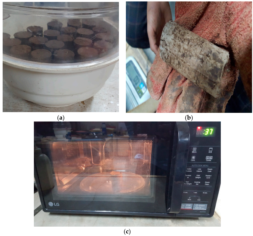
Figure 11. (a) Prepared soil specimens (38 mm dia. and 76 mm height) in desiccator; (b) Dried soil specimens after microwave process; (c) Soil specimens being dried in the microwave oven according to ASTM 4643-8:2008 [1].
