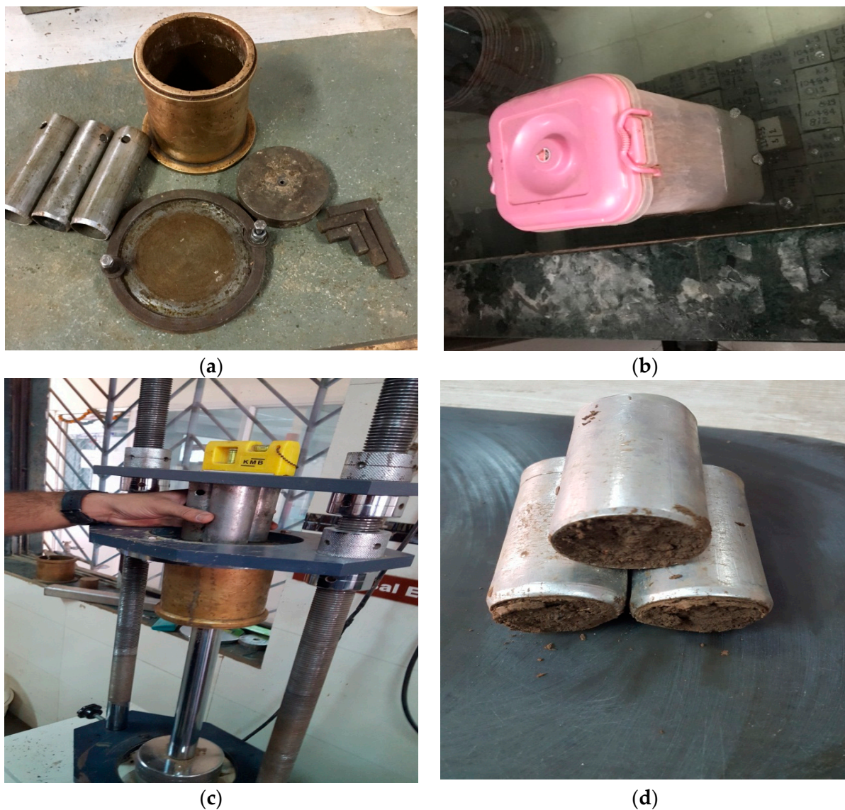
Figure 10. (a) Remolding assembly with layer measurement tool; (b) 24 h soaking of sample prior to casting of specimens under temperature-controlled condition; (c) Specimen extraction by mechanical sample extractor; (d) Three identical soil specimens tested.
