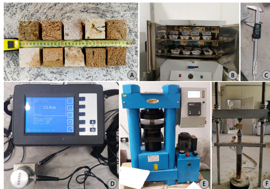
Figure 7. (A) Cubic specimens. (B) Oven at 40 °C. (C) Digital caliper BORLETTI CDJB15 150 mm. Equipment: (D) Matest ultrasonic pulse velocity tester; (E) Matest C070 for uniaxial compression test; (F) point load test.
