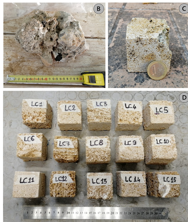
Figure 3. (A) Limestone outcrop belonging to the second-order terrace. (B) Sample CG_3 detail where there is an arenaceous and a calcarenite portion. (C) Detail of the calcarenite portion of the cubic-shaped CG_3 sample. (D) Cubic sandstone and limestone samples subjected to laboratory tests.
