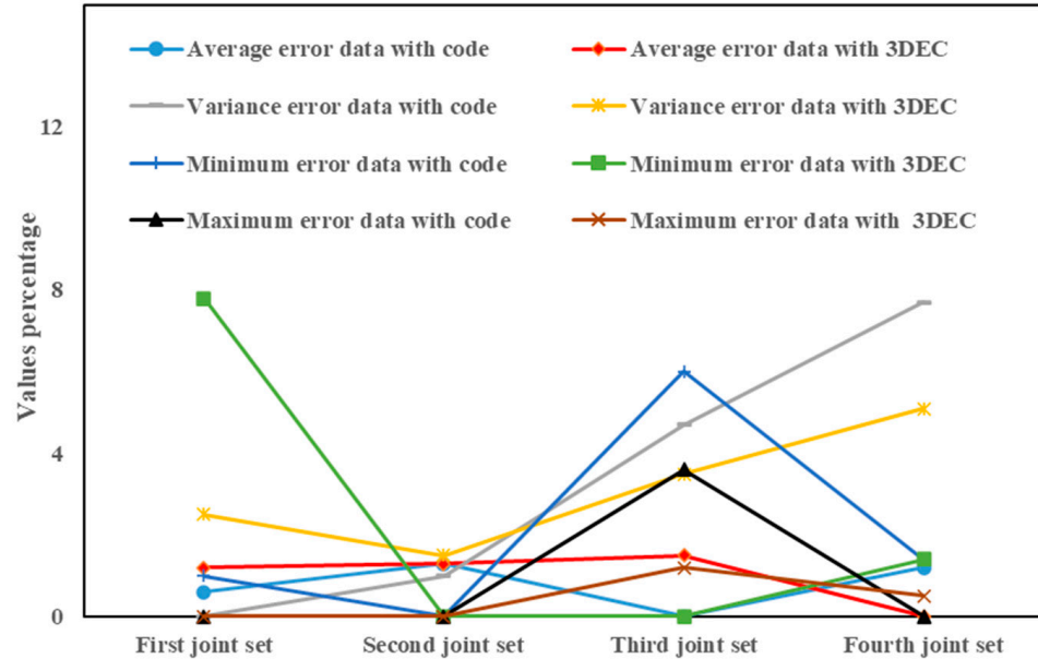
Figure 8. Comparison of the dip calculated via the developed code and 3DEC software with the data obtained from the field survey.
