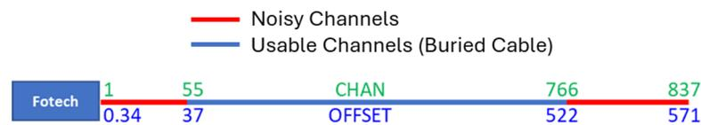
**Figure 4.** Surface DAS geometry assignment.
