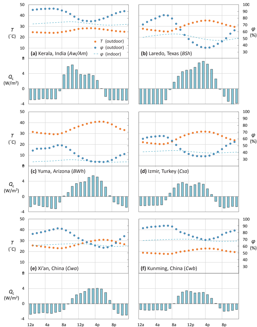
Figure 8. Variation of latent heat flux ( Q_L ; lower panels) and indoor relative humidity ( \phi ; upper panels) with climate in adobe walls. Dots show average hourly July values of outdoor air temperature T (orange) and relative humidity \phi (blue) in each climate (Table 3; (a) Kerala, India; (b) Laredo, Texas; (c) Yuma, Arizona; (d) Izmir, Turkey; (e) Xi'an, China; (f) Kunming, China), dashed lines show indoor relative humidity, and bars show hourly values of Q_L averaged among all orientations (N, S, E, W) in simulations of 20 cm-thick walls of a well-characterized Chinese adobe ([26,77]; Section 3.2.1). Ambient humidity was the only source of moisture.
