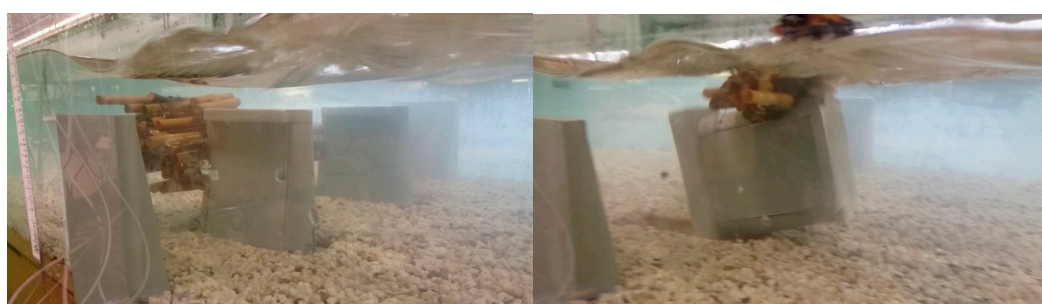
Figure 7. Self-standing pier failure without the deck.
