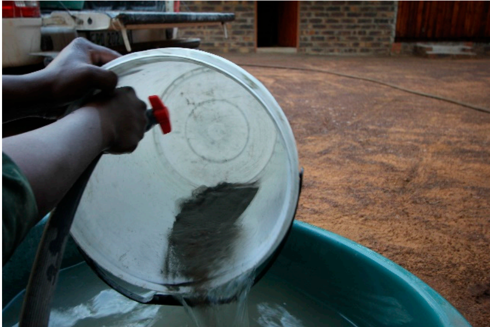
Figure 6. The ‘fast-washing’ process: small amounts of running water are used to wash off the light density material and fines. This process has also been recorded by a covert camera on one of the operations.
