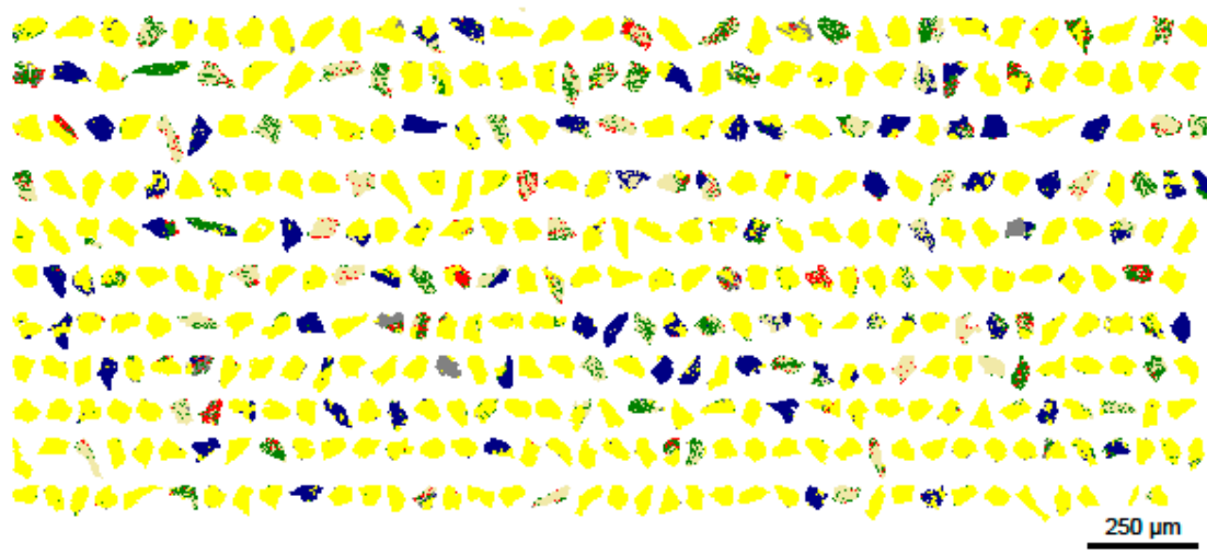
Figure 19. QEMSCAN false-color images of the various mineral particles in the discard of the gravity upgrade. Note that the sulphides (yellow), although liberated, are much finer-grained than those shown in Figure 18 (product prior to upgrading).
