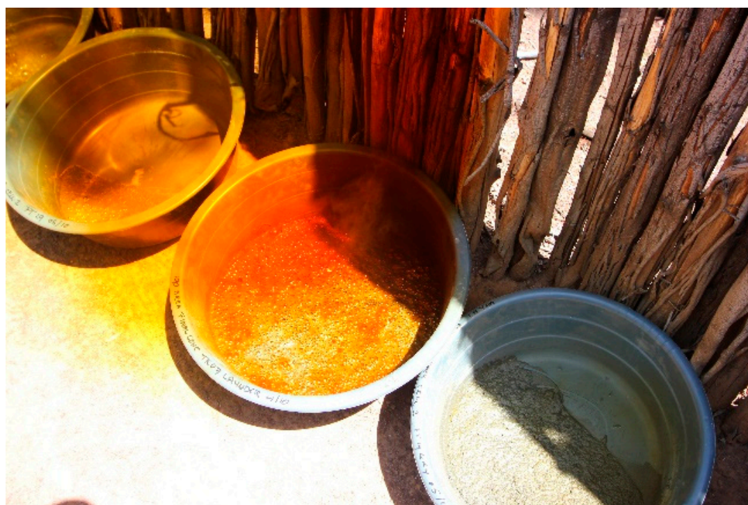
Figure 8. Nitric acid wash: photograph of the reaction of the nitric acid with materials containing abundant sulphides and silicates. Using this nitric acid wash for the illegal upgrading of concentrates is an unsafe practice. Although we applied the same method to replicate the results of this process, the informant was issued with appropriate personal protective equipment.
