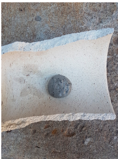
Figure 12. A platinum-rich button—the product of the illicit processing of flotation concentrates. The button is just over 2 cm in diameter.
