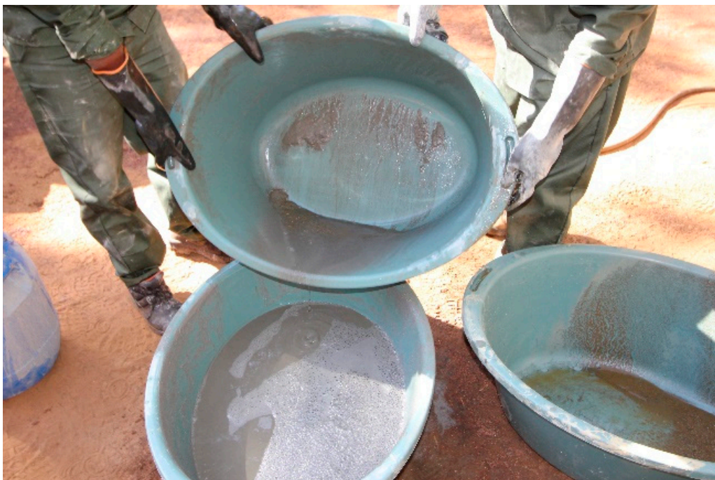
Figure 3. Decanting of the slurry to remove the low-density gangue minerals and fines.
