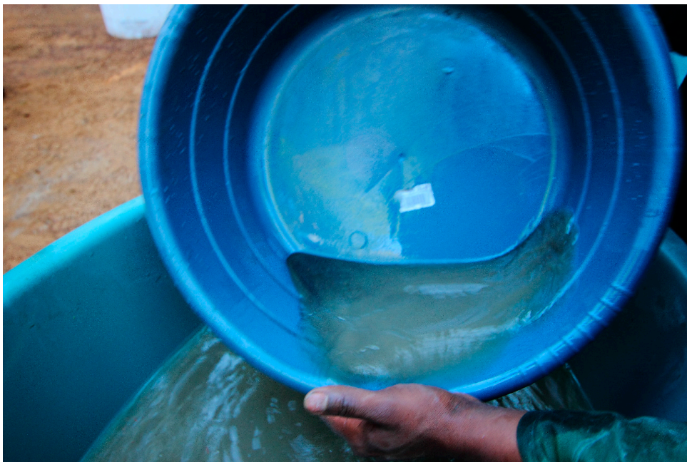
Figure 7. The ‘fast-cleaning’ process. Similar to the ‘fast-washing’ process, this process has also been recorded by a covert camera on one of the operations. Small amounts of water are scooped into the bucket by hand. The contents are then stirred, and the bucket is decanted to remove the lighter material. The water and suspended material are run over the hand for visual inspection.
