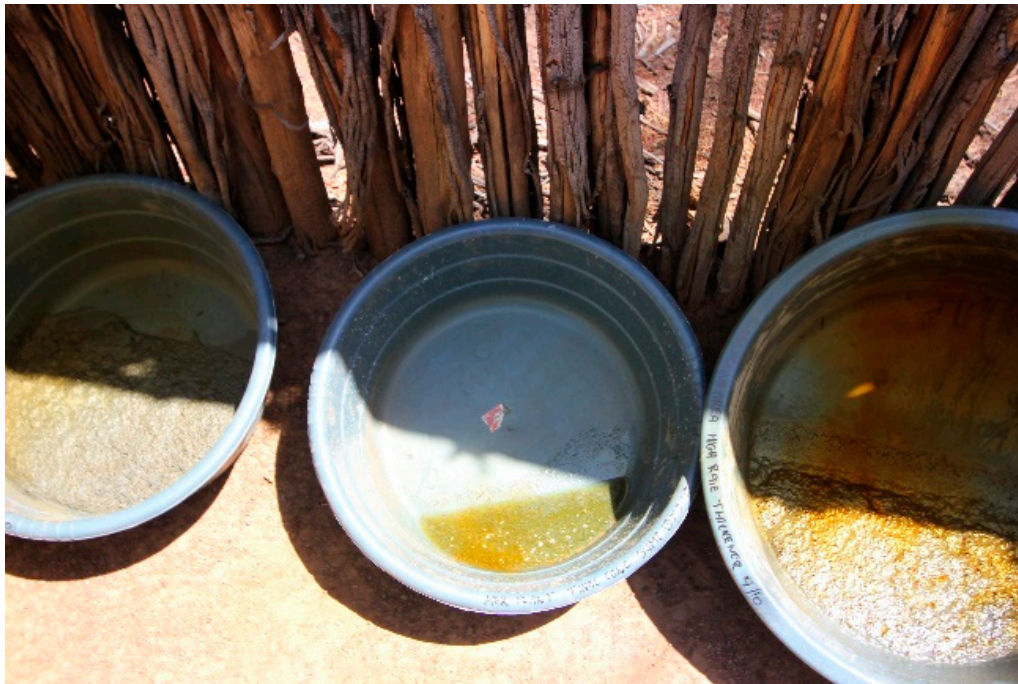
Figure 9. Nitric acid wash: photograph of the reaction of the nitric acid with material containing high levels of chromite and only small amounts of sulphide (middle basin) compared to the reaction with products containing abundant sulphide (to the left and right).
