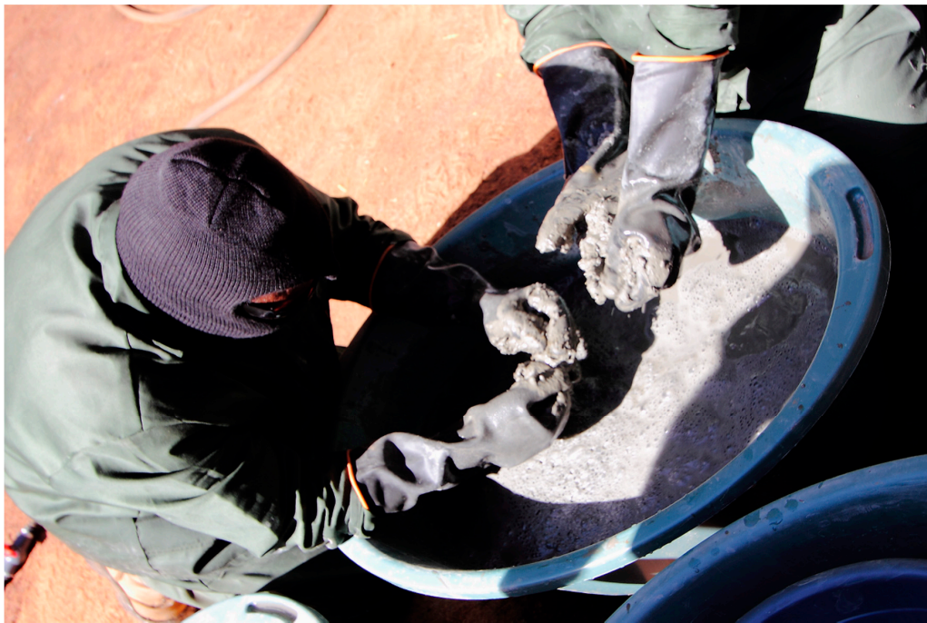
Figure 2. Remixing the material into a slurry and removing some of the plastic, fibers, and woodchips present.
