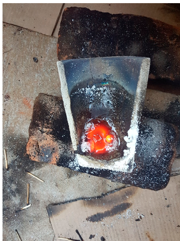
Figure 11. Half crucible containing the molten slag and button just after smelting.
