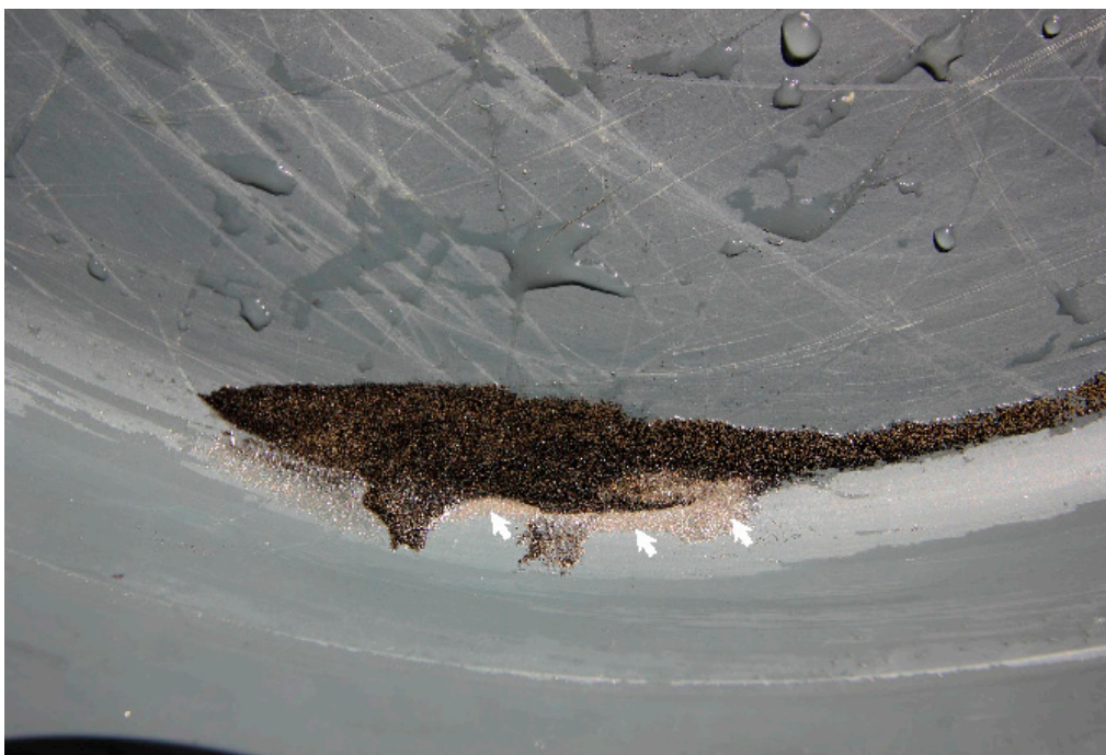
Figure 10. Final product of the washing process. Note the silver streak of the value minerals (arrows). For scale purposes, the photograph is approximately 7 cm in the longest dimension.
