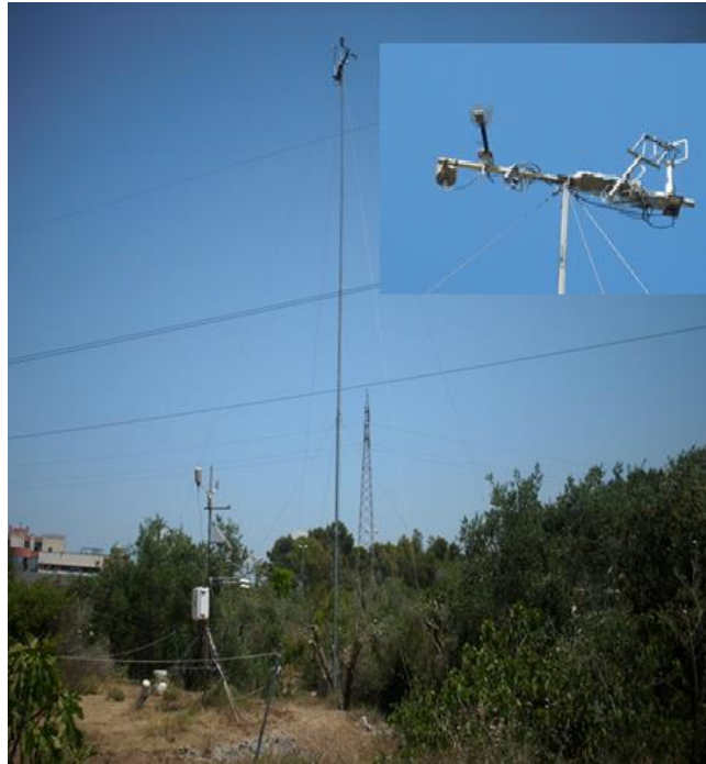
Figure 1. The CNR-ISAC (Consiglio Nazionale delle Ricerche, Istituto di Scienze dell’Atmosfera e del Clima) micrometeorological base; the telescopic mast with a particular of the e.c. instrumentation on top-right, where the Krypton Kh20 hygrometer and the Gill ultrasonic anemometer are visible at the extreme right; the ancillary campbell station collecting the soil data is visible at the bottom left (see also Section 3).
