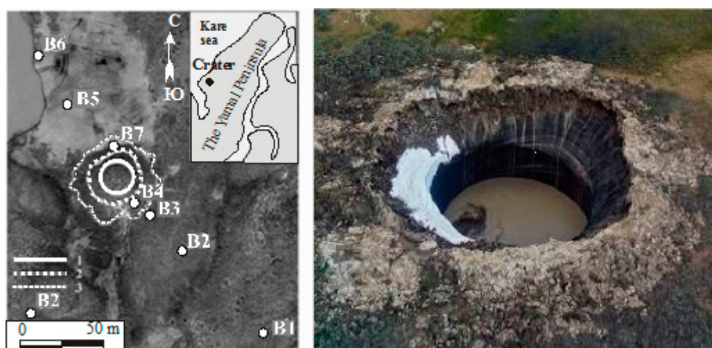
Figure 1. A fragment of a satellite image of the Earth's surface within the Yamal Peninsula indicating the location of the crater (left) and a view of the explosion crater from a helicopter (right). 1, 2, 3 contours: crater vents, explosion funnels, and parapet of parapet, respectively. Named points mark wells and their numbers.
