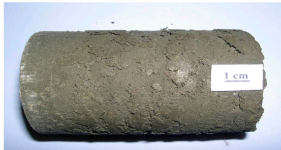
Figure 2. Frozen silty sand with massive (dissemination) pore ice and CH 4 hydrate ( W = 20\% ; K_h = 0.42 ) [18].
