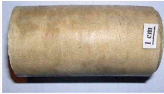
Figure 1. Frozen fine sand-2 with massive (dissemination) pore ice and CH 4 hydrate ( W = 10\% ; K_h = 0.42 ) [18].
