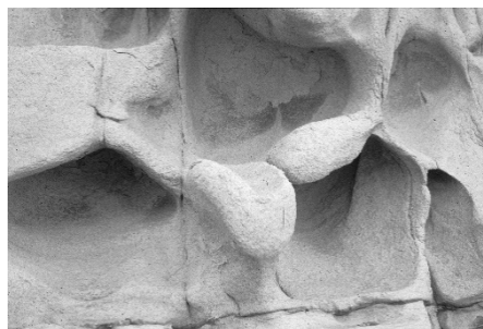
Figure 2. Close-up of some of the tafoni measured. Note the flaked nature of the base of the form suggesting activity rock decay and reduction in the strength of the intact rock.
