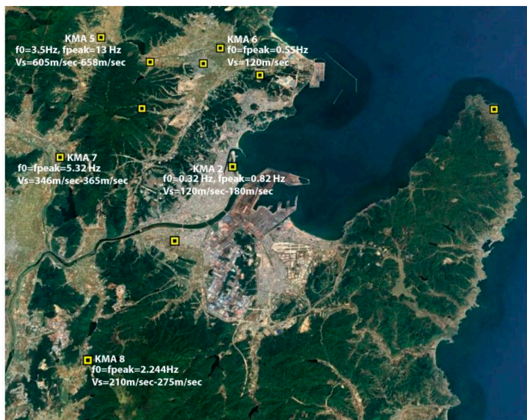
Figure S1. Google Earth Image showing temporary stations installed by KMA around the epicentral area immediately after the earthquake to measure HVSR ratio and understand the subsoil conditions. The yellow square without number indicates temporary stations without any data (modified from [35]).
