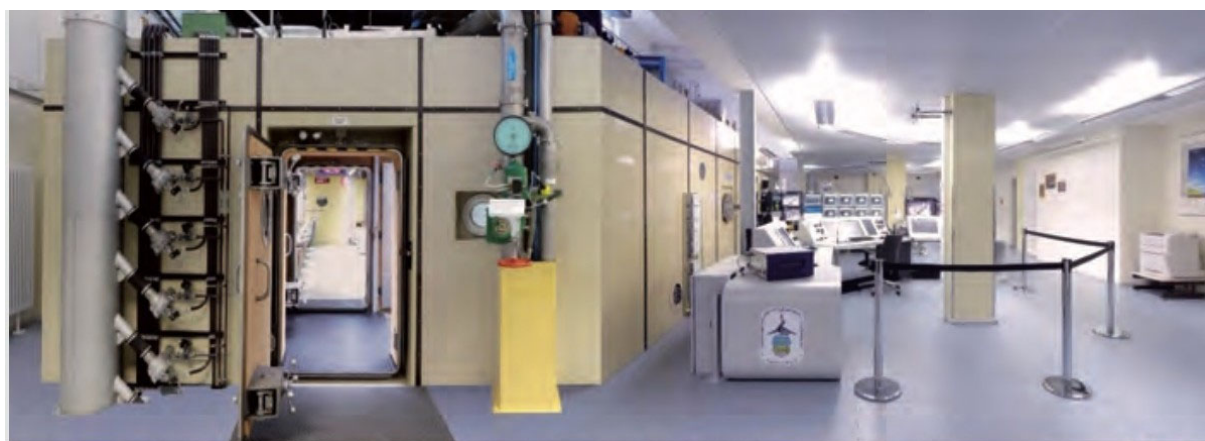
Figure 1. Altitude–climate situation chamber in Königsbrück, with a view of the control station and into the chamber (Source: Senior physician PD Dr. Carla Ledderhos).
