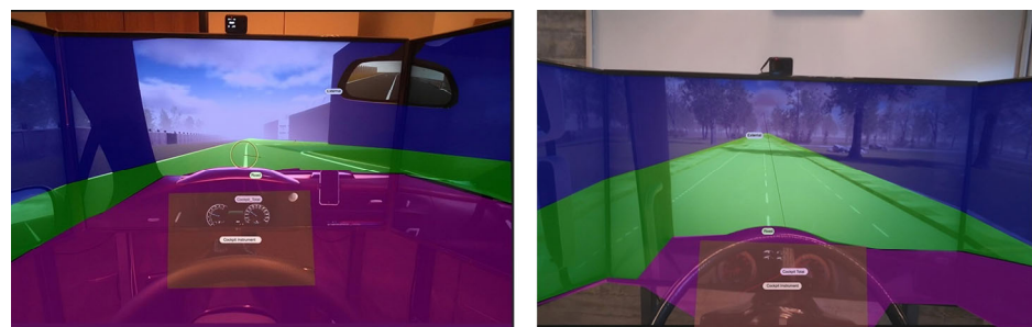
Figure 3. Representation of the AoIs designed for both van ( left ) and truck ( right ) drivers. Green: Road; Orange: Cockpit; Blue: External Environment; Purple: Cockpit Total (this is not discussed in this paper because of the neglectable amount of attention participants paid to this AoI).
