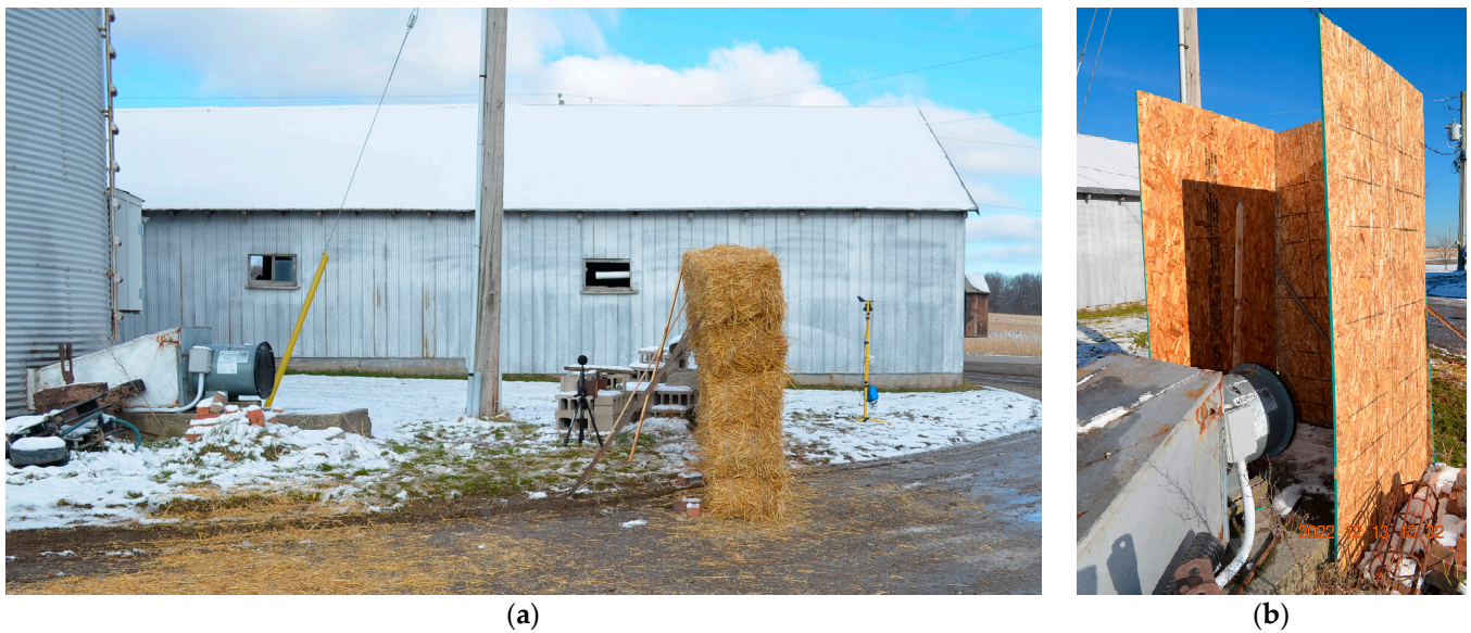
Figure 7. Views of (a) grain bin with fan on left with straw bale barrier in place 4.35 m from fan inlet, and (b) three-sided box enclosing fan inlet.
