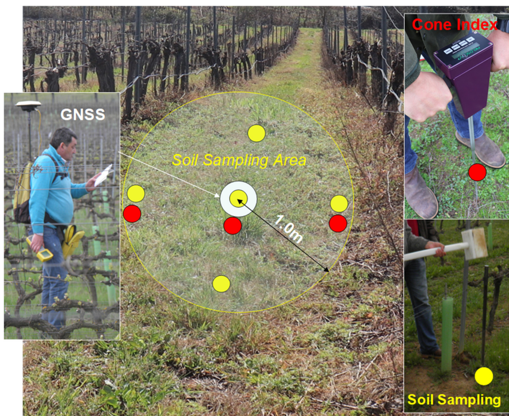
Figure 6. Soil sampling diagram: georeferentiation with global navigation satellite system (GNSS), soil sampling collection and cone index (CI) measurement.
