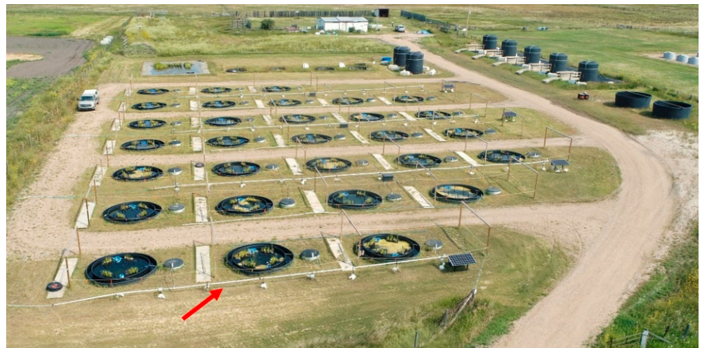
Figure 2. Aquatic mesocosm facility in 2018. Note the presence of wooden walkways and posts near each mesocosm. The dewatering system can be seen as slim white pipes running from one side of the facility to the other (indicated by red arrow).
