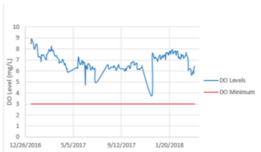
Figure 5.1-1: Aeration Basin Effluent DO Levels Measured Over Time
