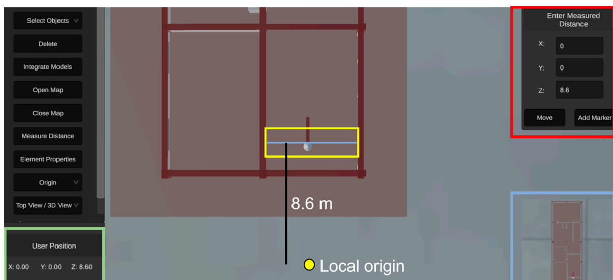
Figure 12. Navigation panel. The pointer in the model moves the distance entered in the panel highlighted in red when the “Move” button is pressed. At coordinate (0, 8.60) m, a glass wall (in yellow) is detected.
