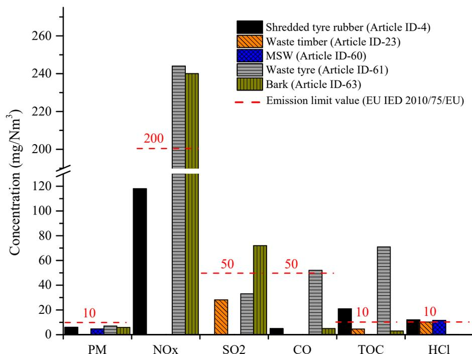
**Figure 3.** Concentration of air pollutants encountered during the pyrolysis of various feedstock after pyrolysis gas burner. The emission limit value (ELV) of air pollutants quoted in the graph is based on the EU IED (2010/75/EU) [28] and is represented by the red dotted lines.
