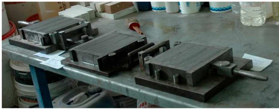
Figure 1. Alkali-activated mortars: casting of prismatic samples for mechanical testing.
