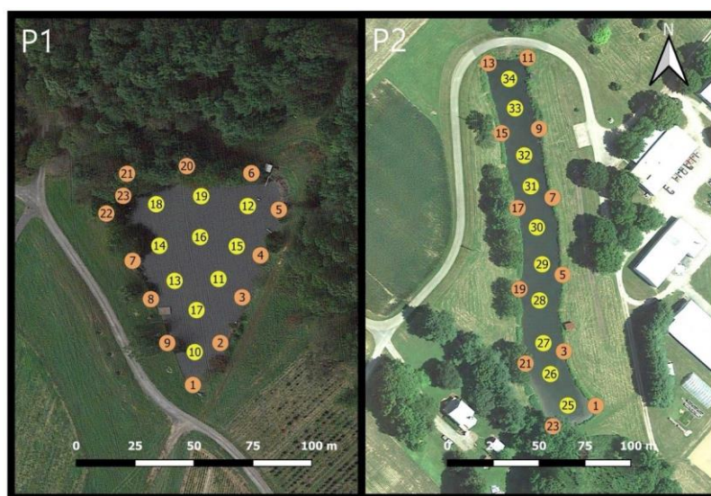
Figure 1. Sampling locations for both Pond 1 (P1) and Pond 2 (P2). Sampling location number is shown inside the circle. Yellow circles indicate interior water sampling locations and orange circles indicate nearshore sampling locations.
