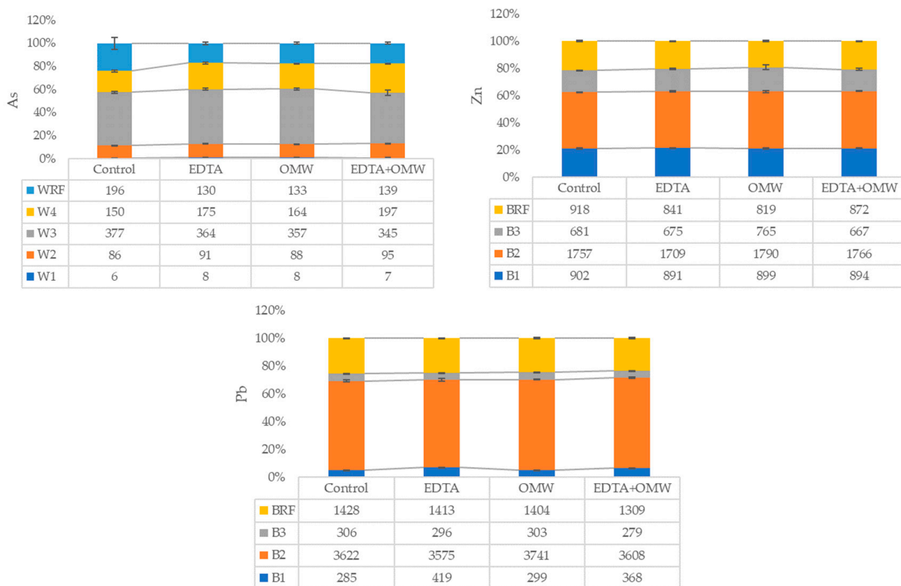
Figure 3. Mean percentages and values of As, Zn and Pb in the different soil fractions, between different treatment schemes (numbers in tables are in \text{mg kg}^{-1} ). The error bars represent the standard error of the mean at the 95% confidence level ( p \leq 0.05 ) ( n = 3 ). W1: nonspecifically sorbed; W2: specifically sorbed; W3: amorphous hydrous-oxide-bound; W4: crystalline hydrous-oxide-bound; WRF: residual fraction; B1: exchangeable/weak acid soluble; B2: reducible; B3: oxidizable; BRF: residual fraction.
