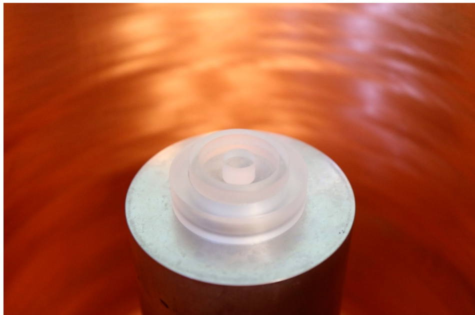
Figure 3. The little jar containing the 4 g of dry residue placed on to the top of HPGe n-type detector.
