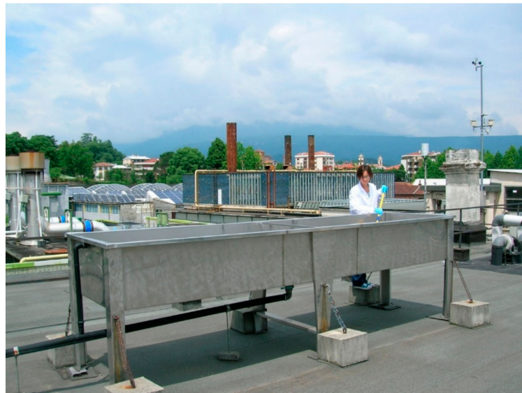
Figure 2. The stainless steel tank placed on the roof of the building for the collection of the wet and dry deposition samples.
