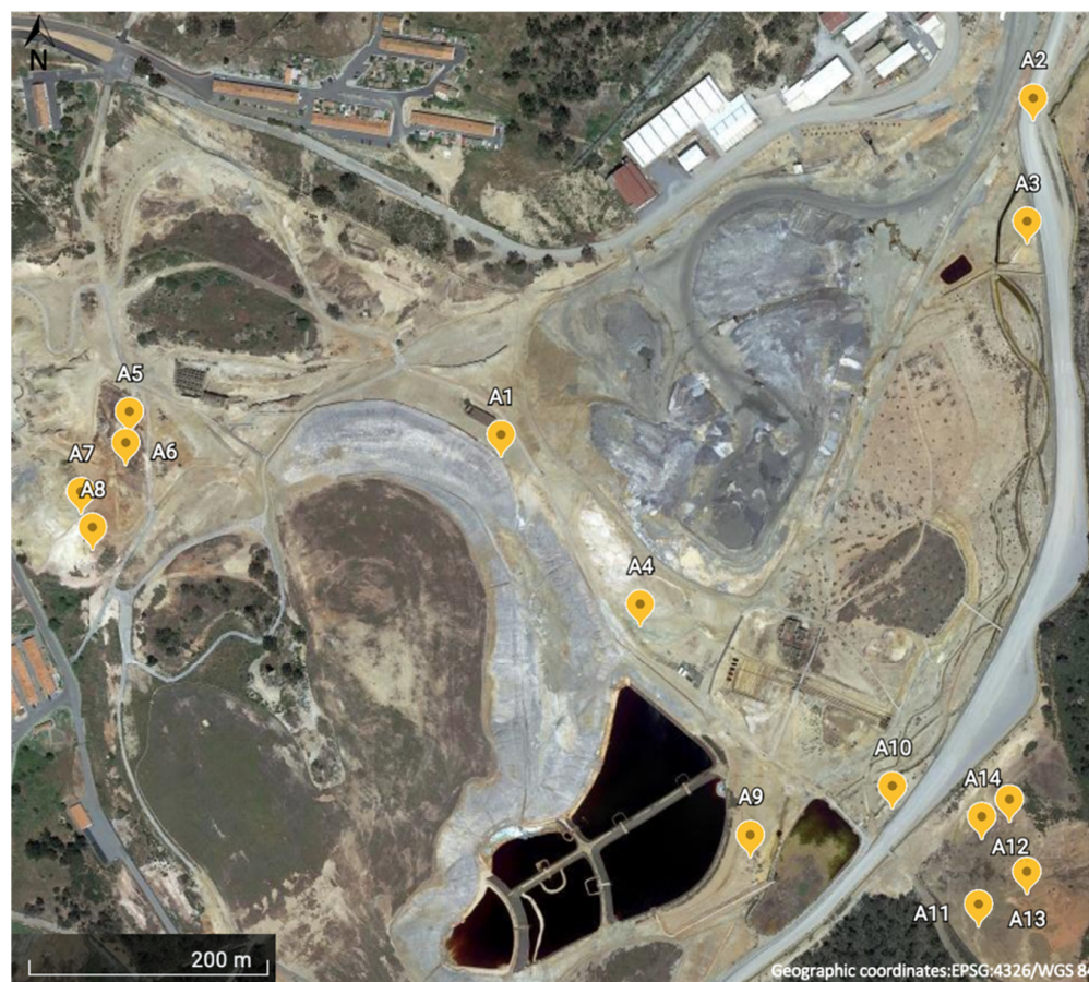
Figure 2. Google Earth image (24 May 2022) evidencing the sampling sites at the Aljustrel mine area, covering an area already rehabilitated by EDM [5]. A1 and A4: sites near the confined waste materials, Algarés area; A2 and A3: sites near the perimetral channels that collect drainage waters; A5–A8: area near recent tailing deposits; A9–A10: soils with scarce vegetation, but eventually representative of natural soils; and A11–A14: soils near old tailing deposits.
