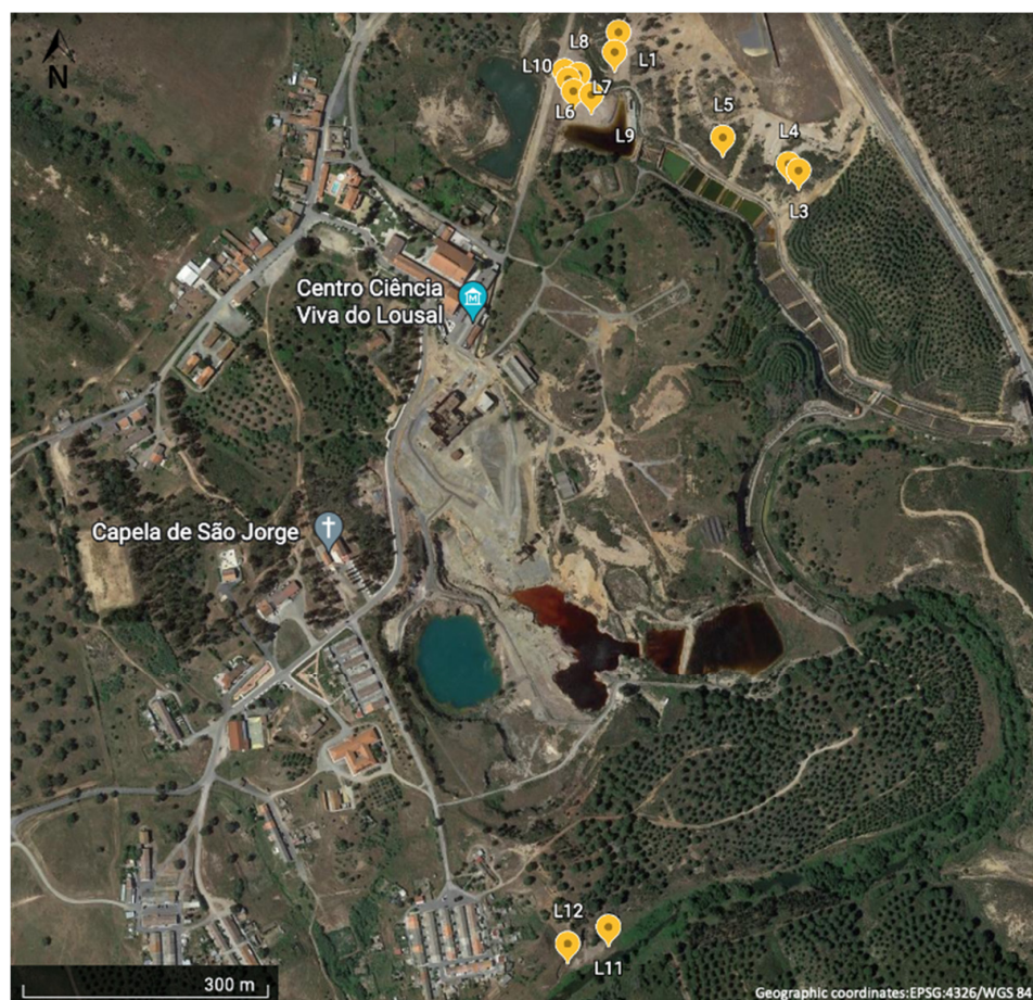
Figure 3. Google Earth image (24 May 2022) evidencing the sampling sites at the Lousal mine area. L1–L5: area potentially affected by acid mine drainage from old tailing deposits; L6–L10; area potentially affected from the pyrite road and railway transport network; and L11–L12: sampling points near the exit of an old mine gallery, with tailing deposits.
