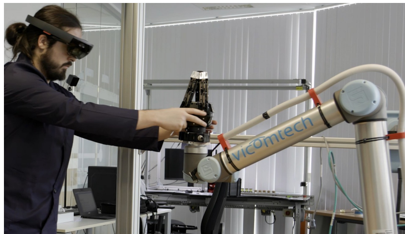
Figure 3. An operator uncoupling the Universal Robot’s Gripper.
