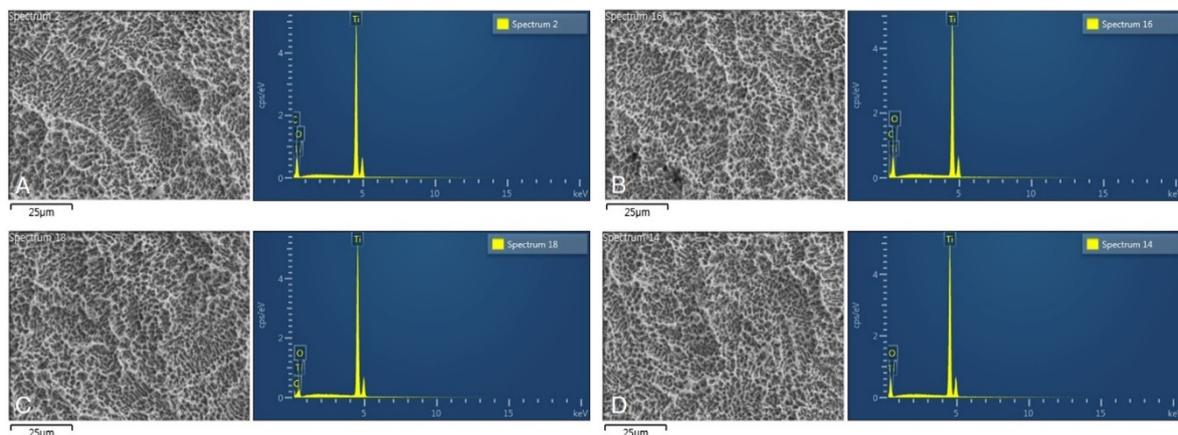
**Figure 4.** Scanning electron microscope (SEM) images and energy-dispersive spectrometry (EDS) analyses of SLA titanium surfaces irradiated with various types of lasers and nonirradiated specimens: (A) control specimen, (B) specimen irradiated with K2 mobile laser, (C) Epic 10<sup>TM</sup> laser, and (D) Saeshin laser.
