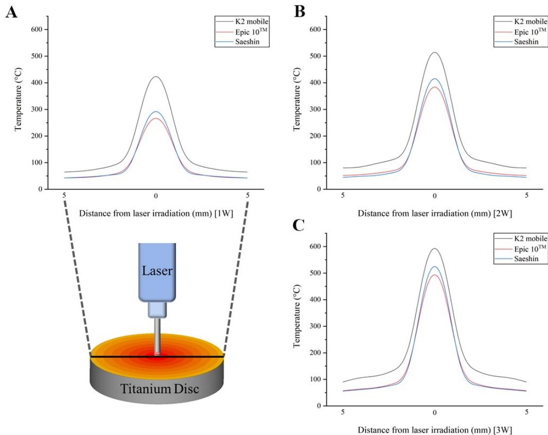
**Figure 2.** Comparison of temperature after laser irradiation using three types of dental diode lasers. (A) 1W, (B) 2W, (C) 3W.
