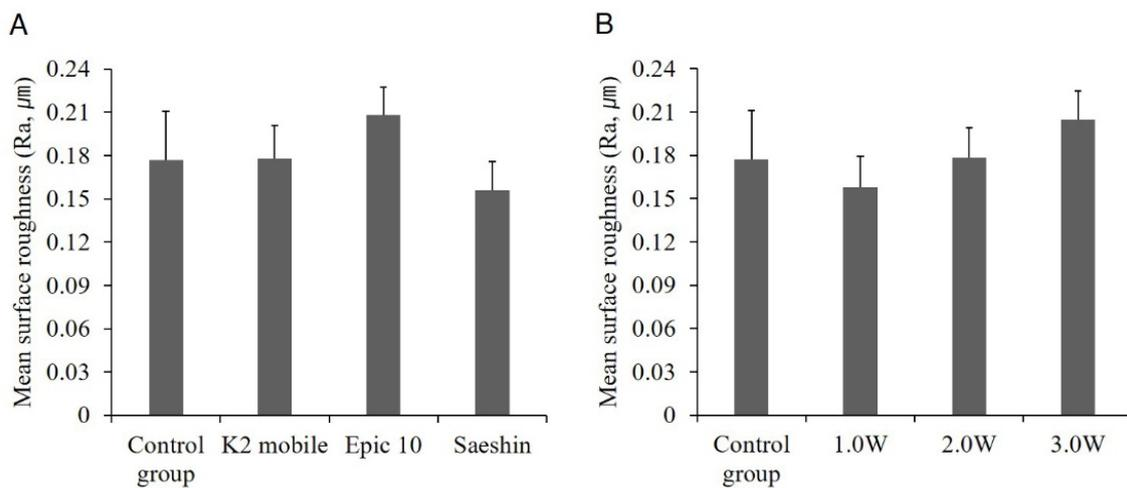
**Figure 3.** Bar diagrams showing the difference in mean surface roughness (Ra) values according to laser types and output powers: (A) a comparison of mean Ra values between various laser types, (B) a comparison of mean Ra values between various output powers.
