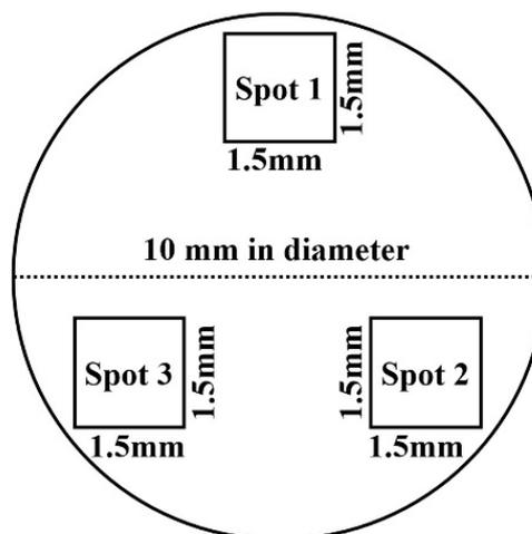
**Figure 1.** Schematic illustration showing three laser irradiation spots on one specimen.
