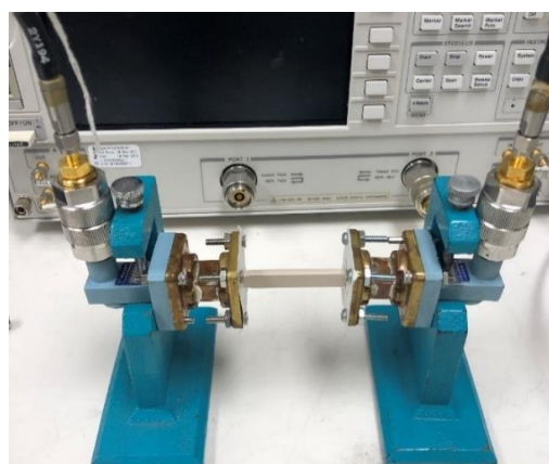
Figure 3. Measurement set up for printed dielectric waveguide.
