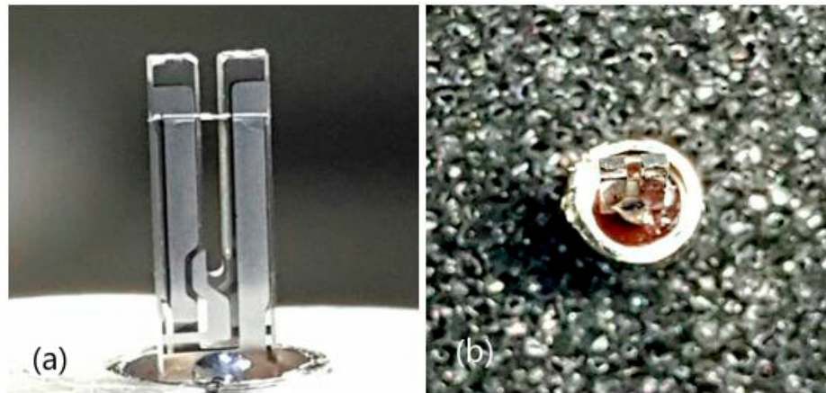
Figure 1. Photograph of a quartz tuning fork (QTF) with polymer microwire bridged across its prongs under a 45× stereomicroscope: (a) front view, (b) top view.
