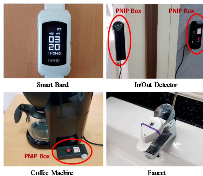
Figure 11. Smart band and proximity-based neighbor identification protocol (PNIP) box.
