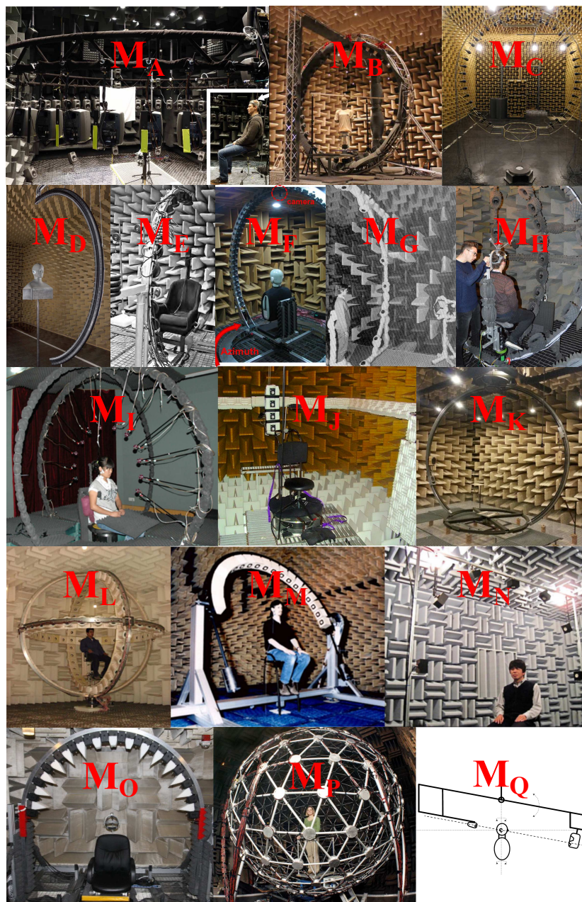
Figure 8. Examples of multi-loudspeaker-based HRTF measurement setups taken from [2,108,116,121–134] (All pictures are taken from available publications, some of them are partly cropped to fit into the overall picture).
