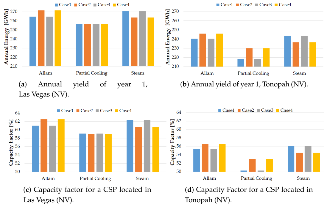
Figure 7. Annual yield and capacity factor for the three power cycles and two locations considered. Designation of cases is explained in Table 6.
