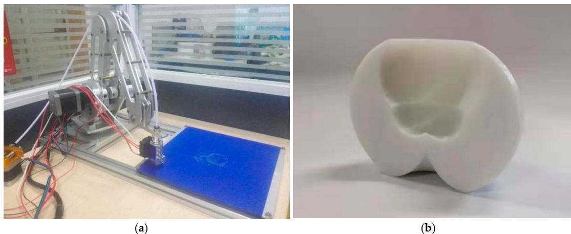
Figure 15. (a) The 3D-printing system robot; (b) a 3D-printed object of the workspace.
