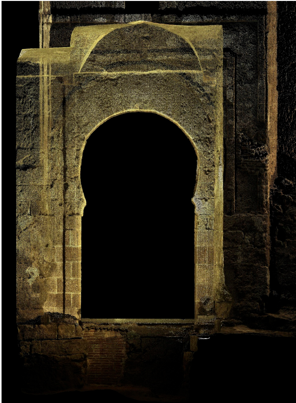
Figure 6. Orthoimage obtained from the point-cloud.
