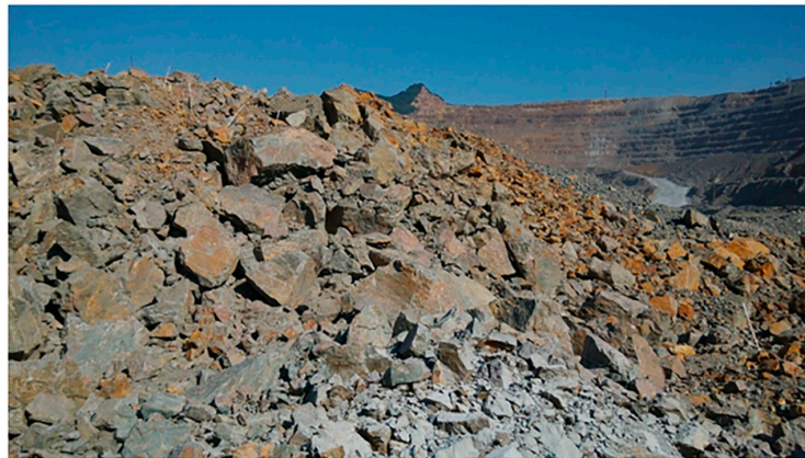
Figure 8. Muck pile on site.
