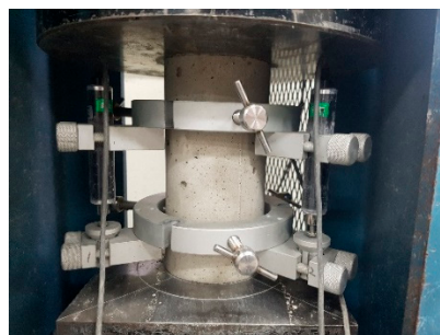
Figure 1. Experimental setup for static destructive test.
