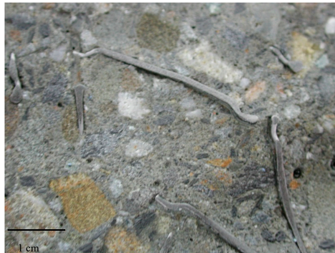
Figure 4. Typical abrasion site in steel fiber concrete abraded by friction abrasive action ( w/cm = 0.36 , ASTM C1138).
