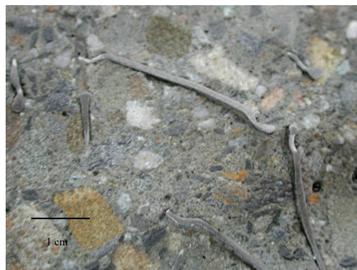
Figure 3. Concrete surface at the end of 72 h of testing (w/cm = 0.50, ASTM C1138).
