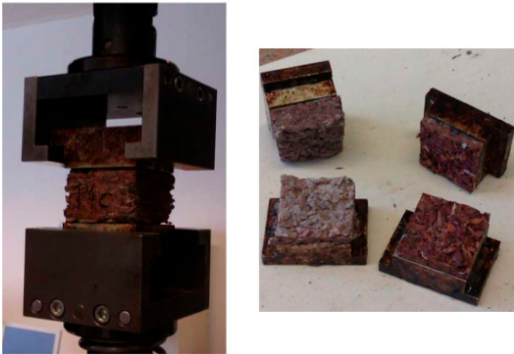
Figure 1. Internal bond test of one sample with larch bark bonded with clay ( left ) and two tested samples bonded with clay and urea-formaldehyde ( right ).
