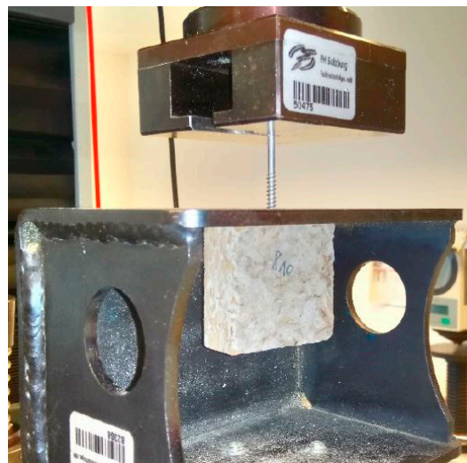
Figure 2. Screw withdrawal resistance of a bark clay sample tested on the edge.
