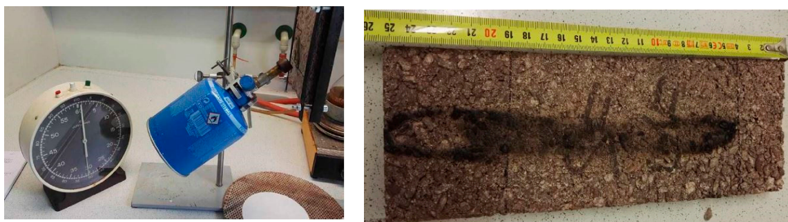
Figure 3. Experimental setup for the small flame test ( left ) and the tested sample ( right ).
