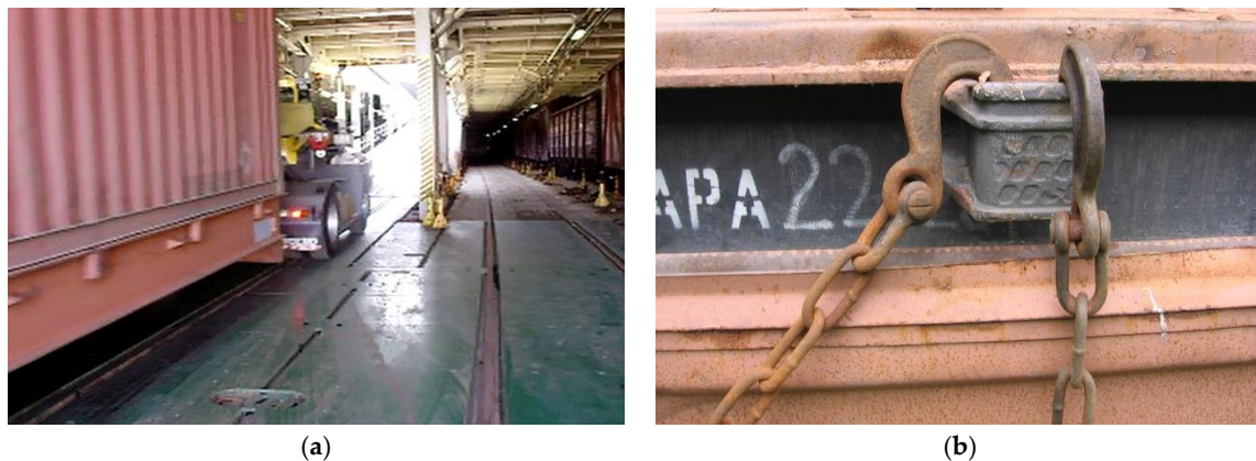
Figure 1. Combined transport trains (a) rolling of combined trains onto a rail ferry; (b) fastening a container train on the deck of a railway ferry.
