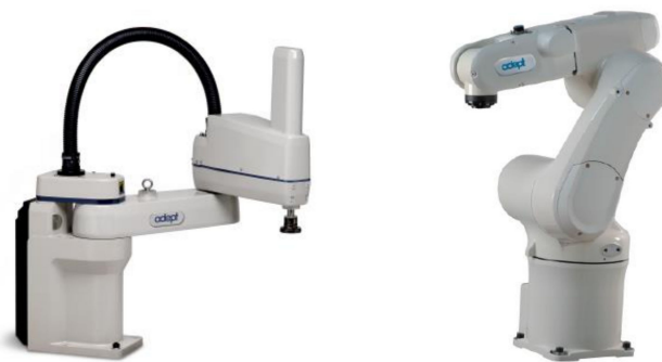
Figure 1. The Selective Compliance Assembly Robot Arm (SCARA) robot ( left ) and the articulated robot ( right ) exploited for the experimental validation of the Kinematic Directional Index (KDI) index.
