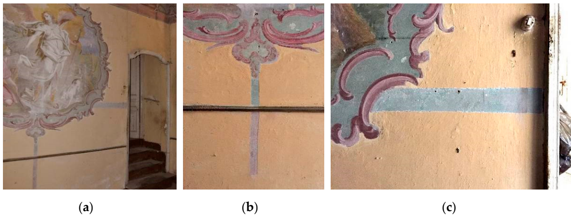
Figure 11. (a) Test performed in the second room (wall with San Giovanni Battista: vertical strip of 100 \times 6 cm), (b) detail of the test with different plaster coloring in the lower and upper parts of the wooden molding and (c) test performed in the second room (wall with San Giovanni Battista: horizontal strip of 100 \times 10 cm).
